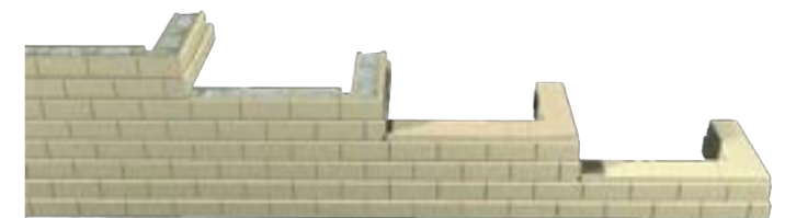
Figure 3: For a step-down that doubles as a planter, turn the wall in 2 or 3 blocks after the AB Corner Block.
