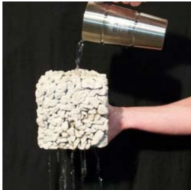
Illustrated: No-Fines Concrete drainage properties
