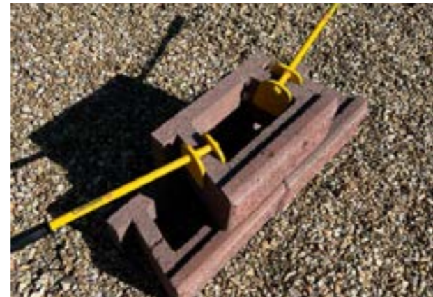
Clamp tool to lift Allan Block®s
